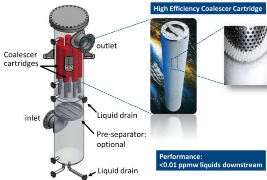
**Figure 2.** A Vertical High Efficiency Liquid/Gas Coalescer
