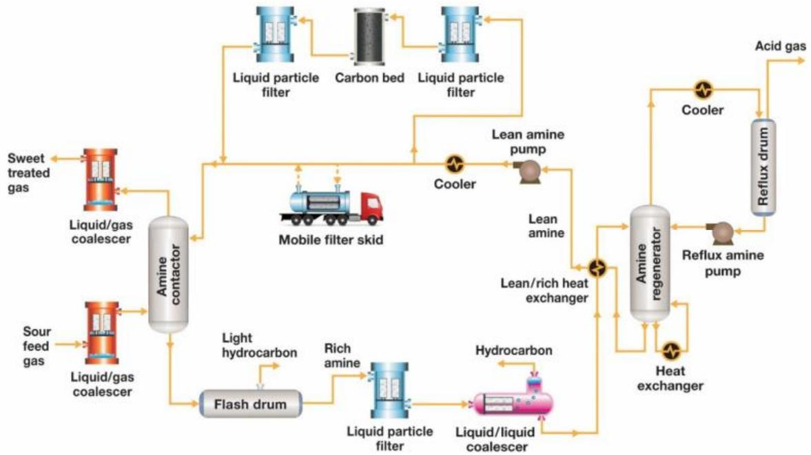
**Figure 1.** Typical Amine Loop Layout with Filtration/Coalescing Recommendations
