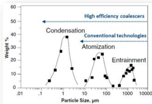
**Figure 3.** Typical Droplet Size Distribution in a Pipe
